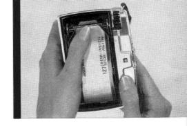
Break and remove the seal on the film and draw the paper across the opening. Insert the tongue of the paper into the longer slot in the take-up spool. Guiding the paper with the thumb of the left hand, turn the winding knob a few turns so the paper is held firmly in place and to make sure the film will wind straight on the take-up spool.
